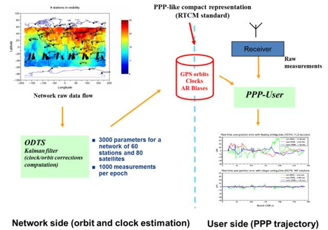
Figure 2: Typical PPP-AR architecture
