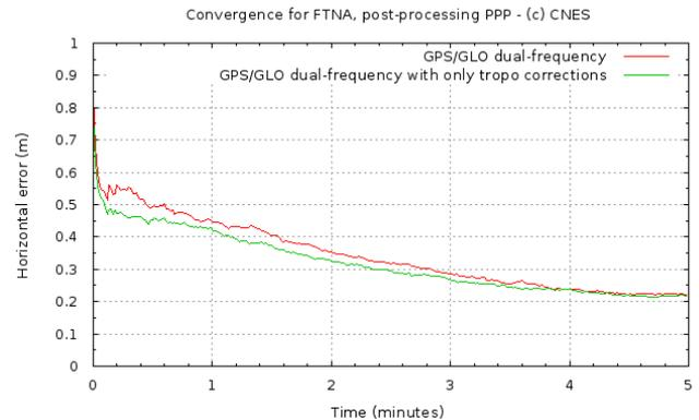
**Figure 14: Comparison with and without troposphere knowledge in dual frequency**
