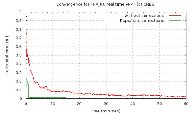
Figure 3: Typical dual-frequency PPP convergence
